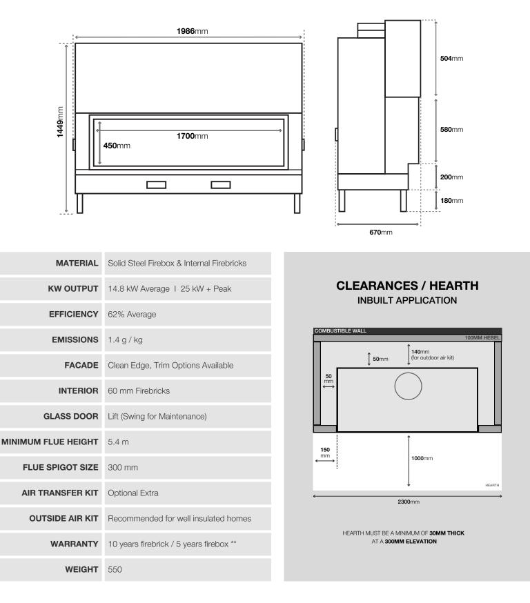
\* Heating capacity of the following appliances are a guide only and refers to areas with 2.4m ceilings and 6 or more star rated buildings. Heating output may vary depending on factors such as characteristics, quality of insulation, type of firewood used and climate zone. \*\* See warranty section in the installation manual for further details. \*\*\* Refer to the Installation Manual for full hearth dimensions and clearances.
